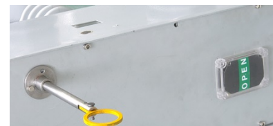
Lockout handle-pulled (open position)
